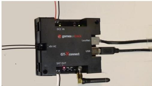
**The GT-Xconnect transmits DCC by Radio as well as positioning information to any radio controller in a car, train, or gaming device. Radio controllers can be integrated with a DCC decoder on one PCB like in the FallerCar system, or they can simply be connected directly to the DCC input of any decoder in a train. The benefit for customers is first of all safe DCC which can**
