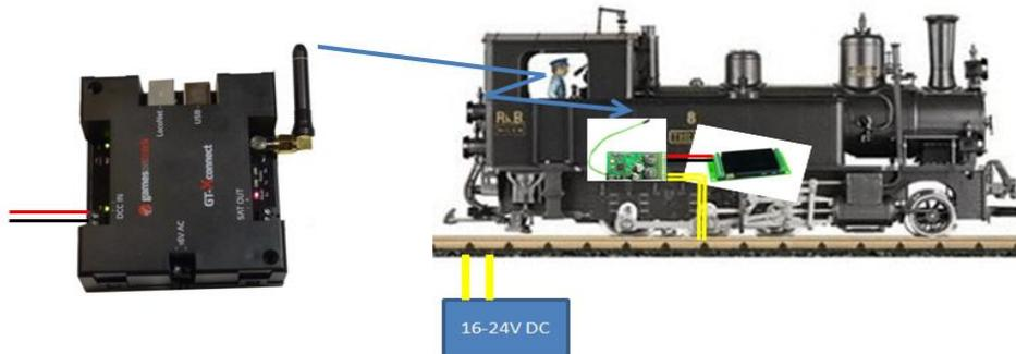
You select a train on your DCC-controller. When you push a command the GT-Xconnect lifts the DCC-signal to the radio and broadcast the signal to any GT-Xcontrol. The GT-Xcontrol captures the signal and push it directly as normal DCC-track power into the decoder. GT-Xcontrol takes power from the tracks. Power can be pure 16-24 V DC or any DCC as well.
