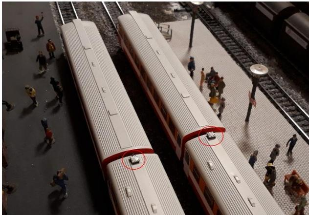
MUST is available as an extension kit with 2 thin wires and a small control electronic to be inserted between the sender platinum and the transducer. It can be mounted through any 1 mm opening in the roof or a crack of any kind. MUST will also be part of any new position senders from GamesOnTrack for tiny trains, cars, and robots.
