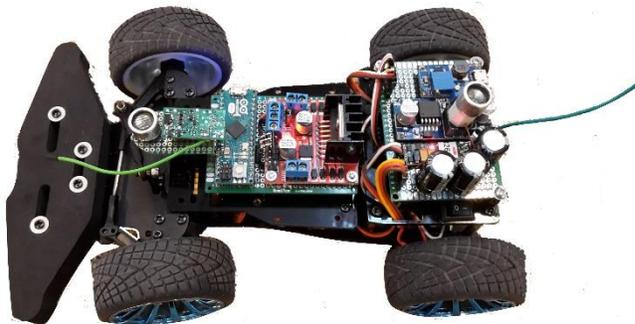
Initially, the Arduino model is meant for cars and trucks in size O/1/G. The principle of an autonomously driven car operating in a free field is useful in many cases. If compared to the Faller Digital Car System, the car is first of all free of wiring, but at the same time it benefits from all the regulation and controls when driving and following a virtual line on
