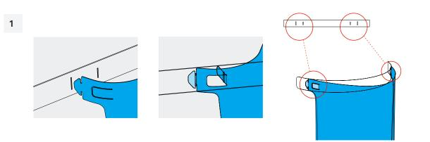
To connect the visor to the fastening strip, insert the ends of the visor into the slits in the strip.
