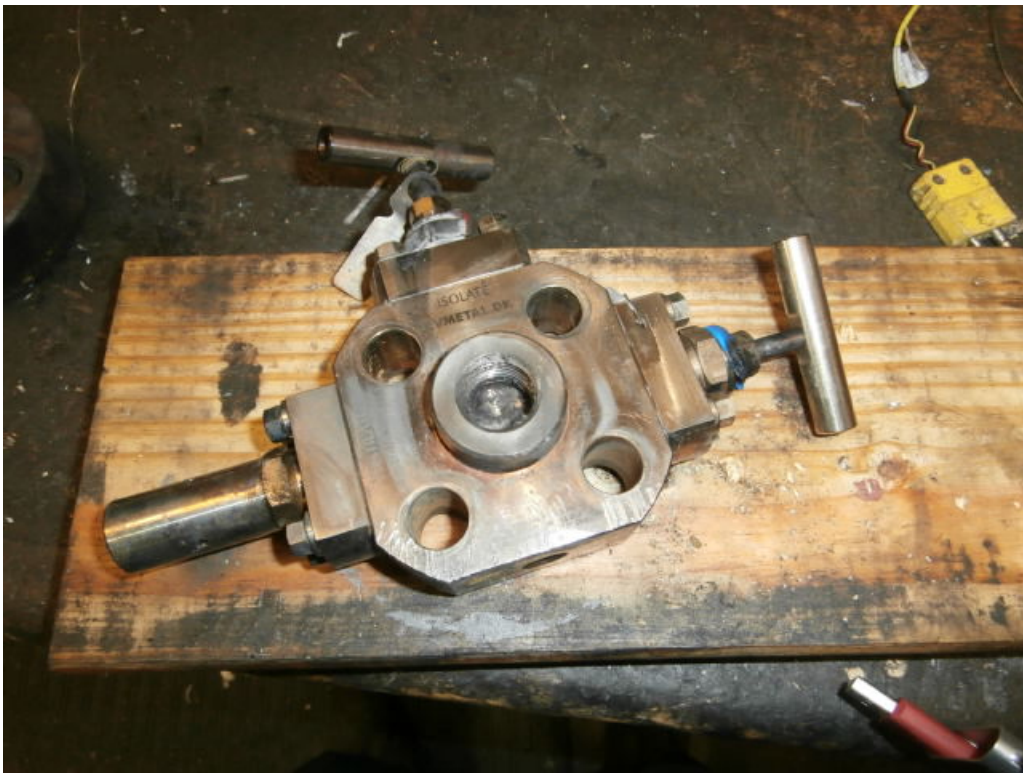
Post-Burn Test Valve
