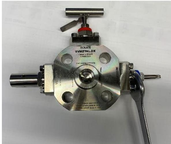
3. Tighten the stem sealing by turning the gland clock wise using a 13 mm key. Note, use a closed key to avoid damaging the hexagon.
