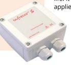
The HLPSS4 4kW controller provides energy saving when used with infrared heaters and also prolongs the lamps' life. It does this by soft-starting the load when power is first applied to the heater(s).
