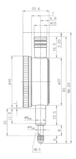
On request we can supply Dial Gauge KM 4 S with threaded protective sleeve and with special transmission ratio range per revolution = 1 mm.
