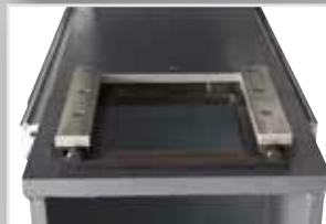
Die holder, tool change also possible with fitted control cabinet door
