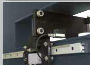
Path measurement of X and Y travel
