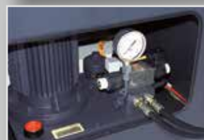
Dual-circuit hydraulic unit in cabinet base
