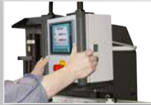
Pivoting control panel with two-hand operation
