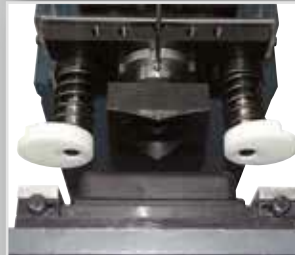
Tool holder, anti-twist in piston rod, hold-down device / scraper combination
