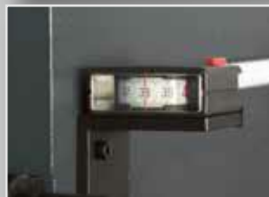
Tape measures display for Y-axis
