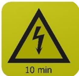
Before opening the electrical panel, disconnect the power connector and lock it to prevent accidental reconnection. Wait 10 minutes after disconnecting the power before accessing the electrical panel, as power is stored in the frequency converters. The panel may only be opened by authorised personnel.
