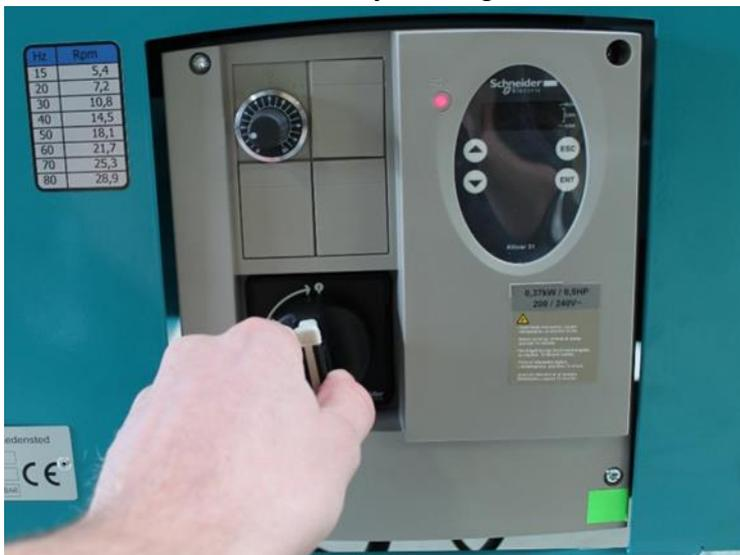
3. Set the drum RPM using the potentiometer. The display shows the current frequency in hertz. Use the table on the left of the control panel to convert this to RPM.
