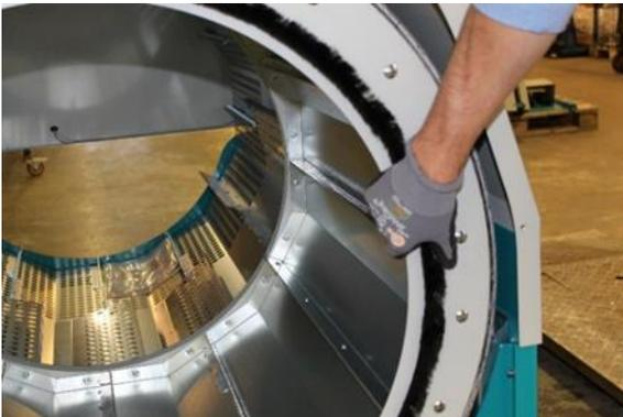
5. Securely tighten the bolts for the tensioning wheel.
