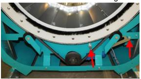
3. Tighten the v-belt so that the drum cannot be lifted out of the guide wheels.
