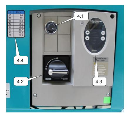
The drum RPM can be adjusted on the control panel by turning the potentiometer (4.1). The drum RPM can be found in the table (4.4) based on the frequency shown on the display (4.3).
