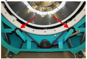
**4.** Check the v-belt has been correctly tightened by starting the engine at 20 Hz and holding the drum. The v-belt must not slip on the drum. **Remember to use gloves!**
