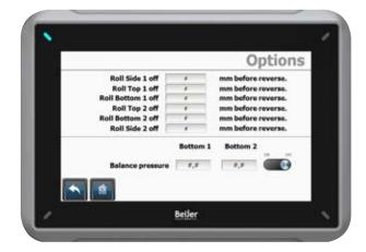
Use this menu to adjust how far the individual scraping rollers are to scrape the skin before they cut out. The length refers to the distance (in mm) from the point where the beam is fully inserted to the point where the rollers are to cut out.
