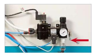
The machine requires compressor pressure of at least 7 bar and an air flow of at least 230 litres per minute when operating at 230 skins per hour. Use a type Cejn 320 coupling to connect the air supply.
