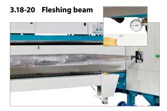
The fleshing beam is heated to a temperature of between 32 °C and 38 °C. The support roller ensures that the beam remains stable while the top rollers are scraping the neck. From the operator's station, you can check the beam temperature at the temperature gauge positioned at an angle behind the fleshing beam.
