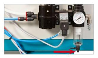
Open the tap to drain the condensation water. Use a suitable container to collect the liquid so that it does not spill onto the floor.
