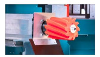
HG recommends that you replace the scraping rollers for every 6,000 skins processed. Unscrew the nut on the end of the roller and remove the washer. Release the scraping roller and replace it with a new one. Replace the washer and nut, and securely tighten the nut. Replace the nut as required.
