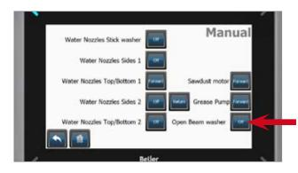
The "Cannot start – beam washer opened manually" alarm appears, access the "Manual" menu and deactivate the "Open beam washer" function.
