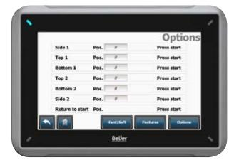
This menu provides assistance with adjusting the scraping rollers.
