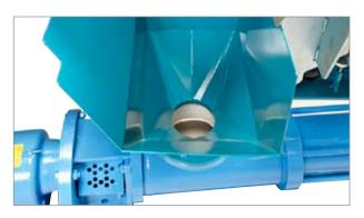
The fat falls into the fat pump, which can transport it over a distance of up to 40 metres. Fit a fire hose between the fat discharge and the fat container.
