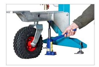
Use a jack to lift the machine's legs one by one. Fit the wheels into the purpose-built holes in the legs. Secure the wheel axle using a washer and bolt, and then lower the jack so that the leg rests on the wheel. Once the machine has been manoeuvred into position, reverse the process to remove the wheels one at a time.
