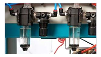
The two glass containers for filling lubrication oil are mounted behind the machine. Gently press the glass container upwards and unscrew it. Use mist lubrication oil.
