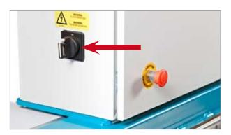
When the main switch is set to <OFF>, there is no power connected to the machine. Turn the switch to <ON> when you want to operate the machine. You must make sure to lock the main switch in the <OFF> position when performing repairs or maintenance on the machine.
