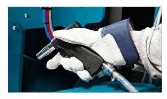
The hot water pistol is used for cleaning funnels and the fat pump. **NB:** Always wear gloves when using the pistol. The water temperature is approx. 60 °C, which is hot enough to cause burns to exposed skin.
