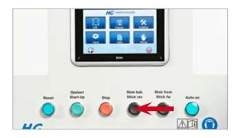
The machine cannot start because the beam is not in its starting position. Use the <Stick rev.> button to return the beam to its starting position.
