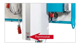
The thermostat for setting the water temperature in the spray system is mounted on the water heater. Set the thermostat at 60  $^{\circ}$ C (approx. "7 o'clock" on the dial) and wait until the water reaches the right temperature. When the water heater is switched on, the red light below the thermostat will be illuminated.
