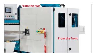
You can access the eight scraping rollers from three sides of the machine. For safety reasons, you cannot use the machine for scraping until all the access routes to the scraping rollers have been closed correctly. Therefore, it is essential that you know where and how to open and close the doors.
