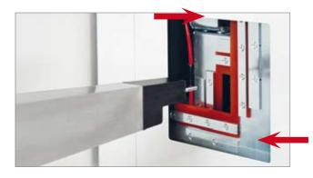
The "Beam washer, vertical not up" and "Beam washer, horizontal not out" appear if the beam washer sides are not open when they should be. Press <Stop>, remove the front panel from the beam washer and check the sensors. (The arrows indicate where the sensors are positioned behind the panel).
