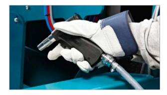
Use the compressed air pistol to remove fur and dirt from around the electrical parts of the machine. Use water/petro-leum to clean off fat and grease. **NB** Always wear gloves when using the hot water pistol for cleaning. The temperature of the water in the pistol is  $60\,^{\circ}$ C.
