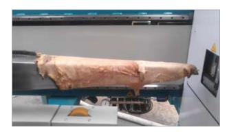
Pull the skin onto the beam with the leather side out and the head at the pointed end of the beam. Stick the two spikes on the front of the beam through the eye holes, and lay the tail on the top side.
