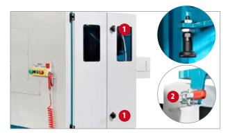
There are handles on all the exterior doors. In addition, there are closing and locking mechanisms in the places indicated here. These principles also apply to the rear access routes.
