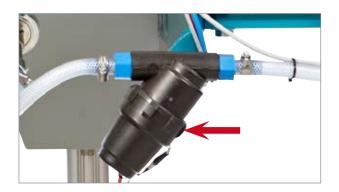
Check the water filter and clean as required. Unscrew the cover to access the filter.
