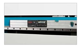
Remove the transport wheels (see Section 2) and adjust the leg height so that the machine is stable and level (both vertically and horizontally).
