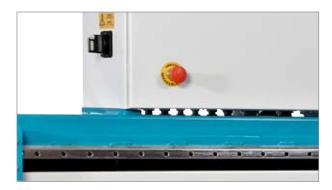
There is an emergency stop button on the start panel and above the fleshing beam on the first electrical cabinet. If an emergency stop button has been activated, turn it clockwise to release it and press <Reset> on the operating panel below the touch display.
