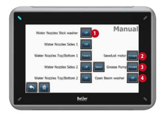
When the machine is in <Stop> status, you can run a number of automatic functions manually.
