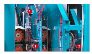
The "Fat scraper, vertical cleaner not out" and "Fat scraper, horizontal cleaner not out" appear if the relevant sensors do not have a "Clear" signal. 1) indicates the position of the sensor for the vertical scraper, and 2) shows the position of the horizontal ones. Press <Stop>, check that there is nothing caught near the sensors and that they are active (illuminated yellow).
