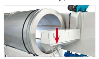
When a throughput drum is used in direct extension to the machine, the drum funnel must be positioned so as to prevent the risk of body parts being crushed between the funnel and the casing containing the skin remover. The shield must be adjusted to match the equipment on site, and additional shields must be added if there are any openings wider than 8 mm.
