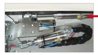
This alarm is triggered if the skin remover fails to open the jaw panels when the beam returns to its starting position. Check whether the sensor is activated when the remover runs backwards and forwards again. Adjust the sensor if necessary.
