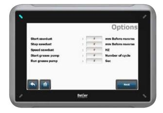
Use this menu to decide how much sawdust to apply, and to choose how often the fat pump is to run. **NB!** Make sure that the pump does not "run dry", as tendons will otherwise have a tendency to stick.
