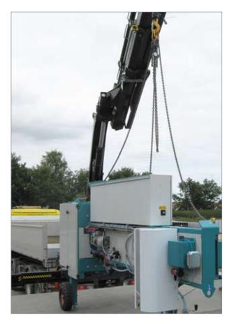
**WARNING!** The machine weighs 1,500 kg and must only be lifted using a crane fitted with approved equipment and operated by persons who have received the appropriate training.
