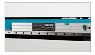
Remove the transport wheels (see Section 2) and adjust the leg height so that the machine is stable and level (both vertically and horizontally).
