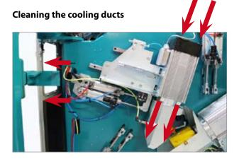
Each of the ten scraping rollers has a separate motor. Every day, use the compressed air pistol to blow any dirt out of the cooling ducts on each motor. Otherwise, there is a risk of the motor overheating.
