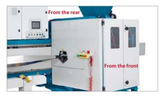
You can access the ten scraping rollers from three sides of the machine. For safety reasons, you cannot use the machine for scraping until all the access routes to the scraping rollers have been closed correctly. Therefore, it is essential that you know where and how to open and close the doors.
