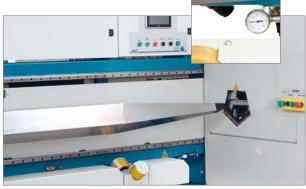
The fleshing beam is heated to a temperature of between 32 °C and 38 °C. The support roller ensures that the beam remains stable while the top rollers are scraping the neck. From the operator's station, you can check the beam temperature at the temperature gauge positioned at an angle behind the fleshing beam.
