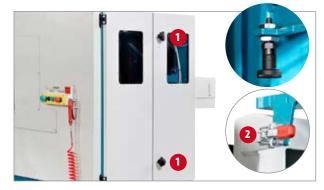
There are handles on all the exterior doors. In addition, there are closing and locking mechanisms in the places indicated here. These principles also apply to the rear access routes.
