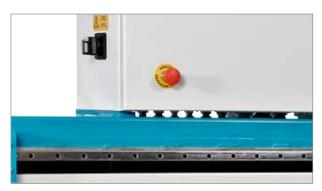
There is an emergency stop button on the start panel and above the fleshing beam on the first electrical cabinet. If an emergency stop button has been activated, turn it clockwise to release it and press <Reset> on the operating panel below the touch display.
