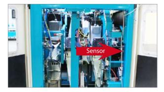
The "Fat scraper, vertical cleaner not out" and "Fat scraper, horizontal cleaner not out" appear if the relevant sensors do not have a "Clear" signal. Press <Stop> and check that there is nothing caught near the sensors and that they are active (illuminated yellow).
