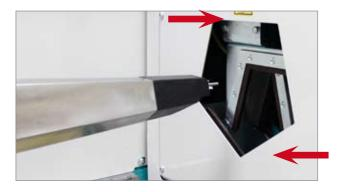
The alarms "Beam washer not open" and "Beam washer not closed" appear if the beam washer sides are not open or closed when they should be. Press <Stop>, remove the front panel from the beam washer and check the sensors. (The arrows indicate where the sensors are positioned behind the panel).
