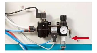
The machine requires compressor pressure of at least 7 bar and an air flow of at least 230 litres per minute when operating at 230 skins per hour. Use a type Cejn 320 coupling to connect the air supply.
