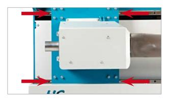
The four lubrication nipples by the fleshing beam are located behind the beam suspension fitting.
