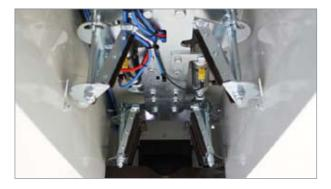
Once the skin has been fully processed, it is automatically removed from the fleshing beam and allowed to drop – directly into a throughput drum, if appropriate.
