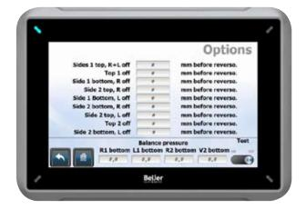
Use this menu to adjust how far the individual scraping rollers are to scrape the skin before they cut out. The length refers to the distance (in mm) from the point where the beam is fully inserted to the point where the rollers are to cut out.
