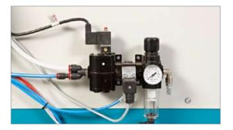
This alarm appears if there is too little air pressure in the machine. Check the air supply.
