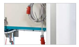
The machine is fitted with three plugs: one 32 A CEE plug and two16 A CEE plug for connecting a 3 x 400 Volt power supply with neutral (N) and earth (PE) conductors. The ground fault circuit breaker (HPFI) must be approved for frequency converters.
