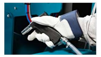
The hot water pistol is used for cleaning funnels and the fat pump. **NB:** Always wear gloves when using the pistol. The water temperature is approx. 60 °C, which is hot enough to cause burns to exposed skin.
