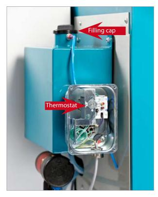
Fill coolant for the beam heating system so that, when cold, there is a gap of 4–5 cm from the surface of the fluid to the top of the boss. Check regularly to make sure that the volume of fluid remains at approximately the same level.
