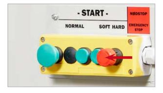
One of the emergency stops has cut out. Reactivate the emergency stop and press <Reset>.
