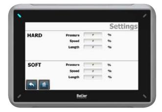
Use this menu to define how the machine is to operate when you use the <SOFT> and <HARD> buttons on the start panel. You can increase or decrease the pressure, speed and length settings and thus adapt the scraping process to match the individual skin types.
