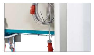
The machine uses three plugs: a 32 A CEE plug and two 16 A CEE plug for connecting a 3 x 400 Volt power supply with neutral (N) and earth (PE) conductors. The ground fault circuit breaker (HPFI) must be approved for frequency converters.
