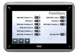
You can use this menu to switch the various automatic functions in the scraping process <ON> and <OFF>. You can also use this menu to check the processes individually.
