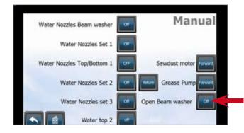
If the "Beam washer manually opened" alarm appears, access the "Manual" menu and deactivate the "Open beam washer" function.
