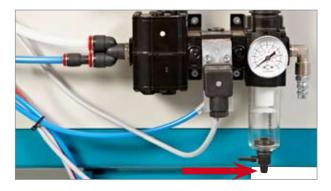
Open the tap to drain the condensation water. Use a suitable container to collect the liquid so that it does not spill onto the floor.
