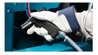
Use the compressed air pistol to remove fur and dirt from around the electrical parts of the machine. Use water/petroleum to clean off fat and grease. **NB** Always wear gloves when using the hot water pistol for cleaning. The temperature of the water in the pistol is 60 °C.
