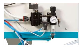
The machine requires compressor pressure of at least 7 bar. Use a type Cejn 320 coupling to connect the air supply. To avoid interruptions to the scraping process, make sure that the air supplied to the machine is free from water, dirt and rust from old pipes.
