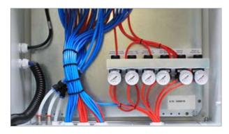
This cabinet contains the compressed air gauges for the beam washer, fat scraper and skin remover. The panel states what is measured where.
