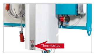
The thermostat for setting the water temperature in the spray system is mounted on the water heater. Set the thermostat at 60 °C (approx. "7 o'clock" on the dial) and wait until the water reaches the right temperature. When the water heater is switched on, the red light below the thermostat will be illuminated.
