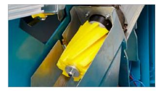
HG recommends that you replace the scraping rollers for every 6,000 skins processed. Unscrew the nut on the end of the roller and remove the washer. Release the scraping roller and replace it with a new one. Replace the washer and nut, and securely tighten the nut. Replace the nut as required.
