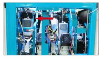
This alarm appears if the sensor has no "Clear" signal. Press <Stop> and check that there is nothing caught near the sensor and that it is active (illuminated yellow).
