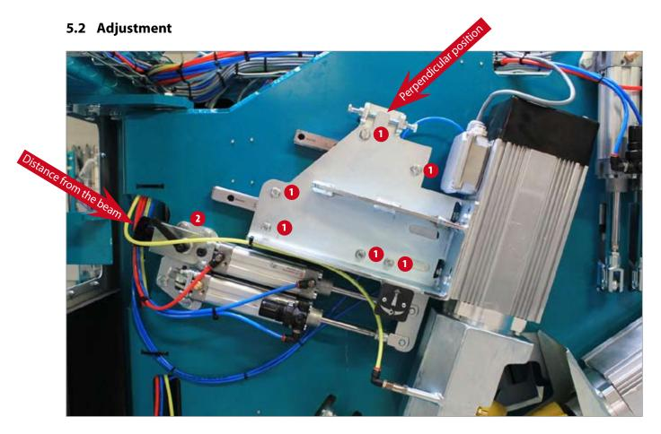
The adjustment process is the same for all ten scraping rollers. You can adjust two aspects:
