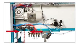
The air line lubricant keeps the machine's bearings lubricated. Press the glass component on the oil container up and turn it anticlockwise. This will release the glass, which you can then top up with oil. Replace the glass component by pressing it up and turning it clockwise.
