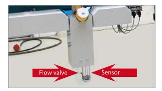
The "Support roll not down" alarm appears if the support roller is not down when it should be. Check the sensor, which you may need to adjust or replace.
