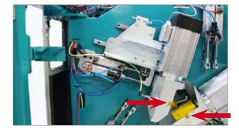
Check the water nozzles at regular intervals. There are six nozzles by the beam washer and one by each scraping roller. Activate the water nozzles manually as described in the "Manual menu" section on page 17.
