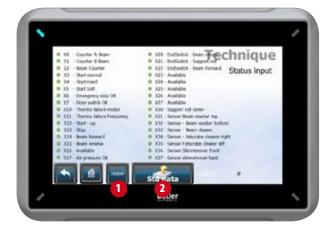
Use this screen to monitor the machine's computer and see the inputs and outputs running to and from the machine. Press (1) to switch to Output.
