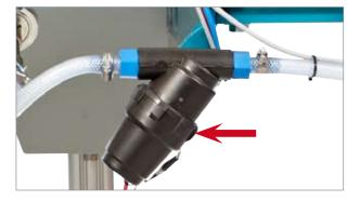
Check the water filter and clean as required. Unscrew the cover to access the filter.
