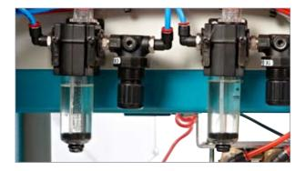
The two glass containers for filling lubrication oil are mounted behind the machine. Gently press the glass container upwards and unscrew it. Use mist lubrication oil.
