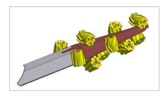
The skin is processed using two sets of five scraping rollers. All ten rollers are sprayed with hot water during the scraping process. This ensures optimal processing and leads the fat away from the skin.
