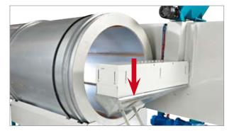
When a throughput drum is used in direct extension to the machine, the drum funnel must be positioned so as to prevent the risk of body parts being crushed between the funnel and the casing containing the skin remover. The shield must be adjusted to match the equipment on site, and additional shields must be added if there are any openings wider than 8 mm.
