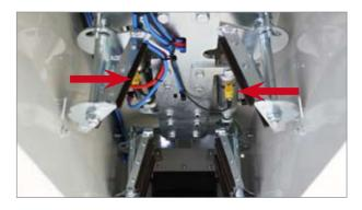
The alarms "Clamp 1 (or 2) skin mover closed" appear if the skin remover is not open when it should be. Press <Stop> and check that the jaw panels are open and that the sensors areactive (il-luminated yellow).
