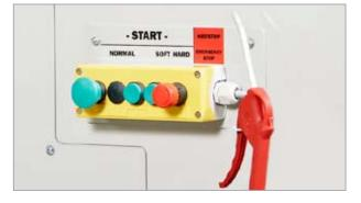
The compressed air pistol is used for cleaning those parts of the machine where it is inappropriate to use water. Wear protective equipment in accordance with the regulations that apply to the use of compressed air.
