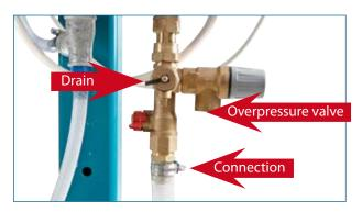
Connect the water heater to a supply of ordinary, cold tap water. To open the water supply, turn the red tap so that the "wings" are vertical. The water heater is fitted with an overpressure valve, which is activated if the water boils. Use the drain valve for frost protection.
