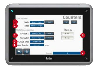
This menu provides an overview of both the day's production and total production for the machine. The menu also shows how many skins have been processed per set of scraping rollers, cycle time and beam counter.
