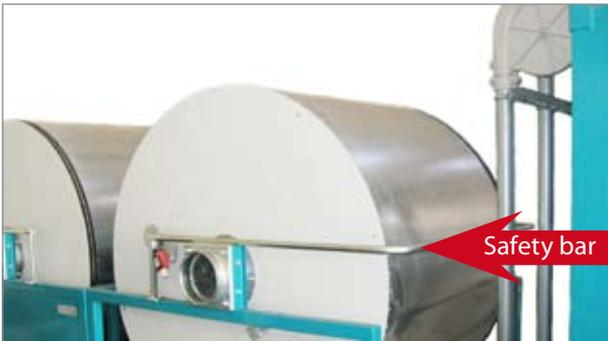
To access the large drums, start by lifting the safety bar up over the drum – this also secures the system against unintentional start-up. Then open the locks at the base of the door, after which the door can be opened. Make sure to secure the door against falling shut before reaching into the drum. When the door is correctly locked and the safety bar is in place once more, the emergency stop can be reset and the system started.
