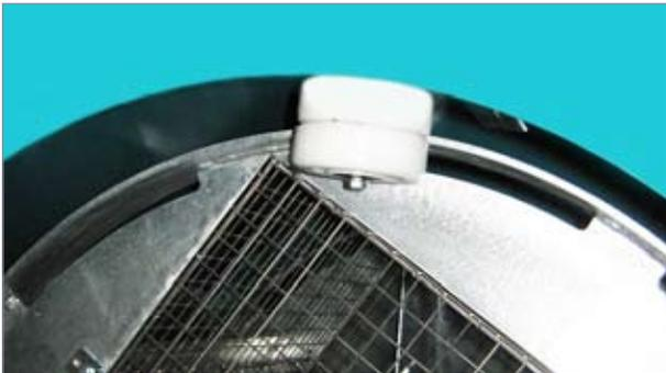
To remove the net drum, start by removing the support wheels at the top. Then simply lift the drum out.
