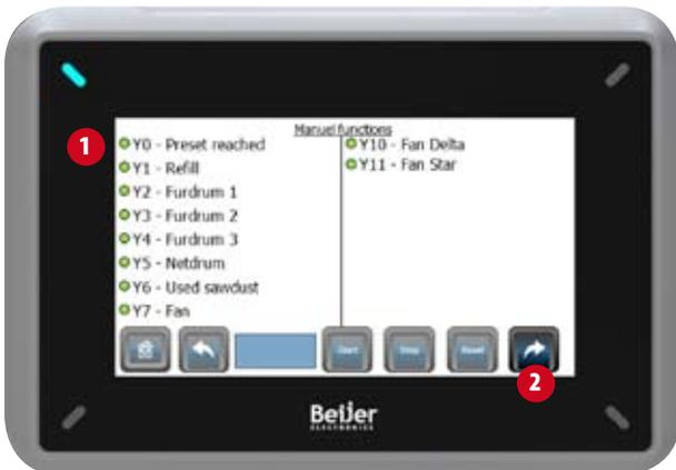
When the machine is in <Stop> status, you can run a variety of automatic functions manually. To start with, press <Stop> on the operating panel and access the menu.
