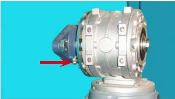
There are four sets of ball bearings on the filter unit: three on the net drum and on the motor located on the back of the unit. Lubricate the bearings with grease before the season starts, and approximately once a week during the season.
