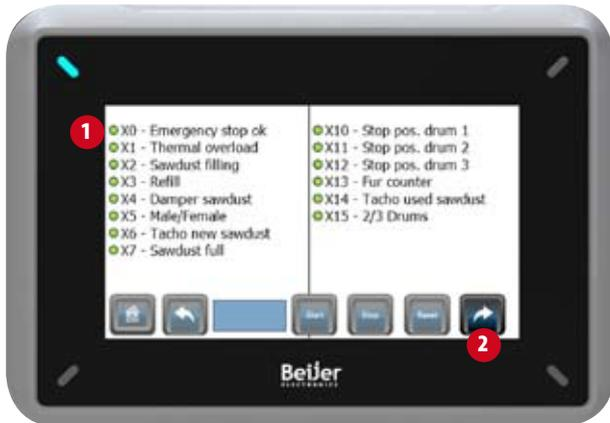
Use this screen to monitor the system's computer and see the inputs and outputs running to and from the machine. The screenshot above shows inputs. The colour of the circle (1) indicates whether the function is active or passive. Green: ON / White: OFF
