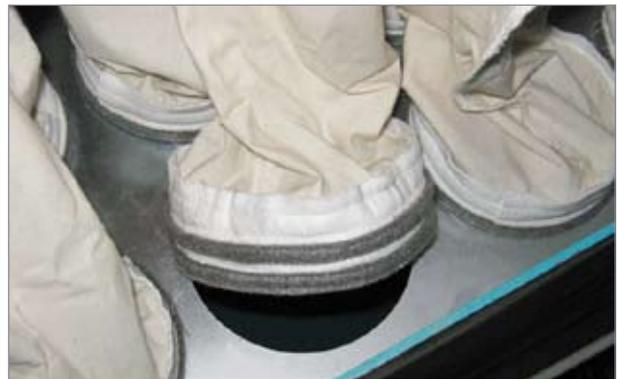
When replacing filters, cut the plastic strip at the top. Then press the collar at the bottom of the filter together and twist it off the panel.
