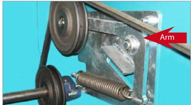
Check the belt tensioner for the net drum as required. It should be possible to turn the arm easily. If the spring has drawn together completely, the belts are too loose and must be replaced.
