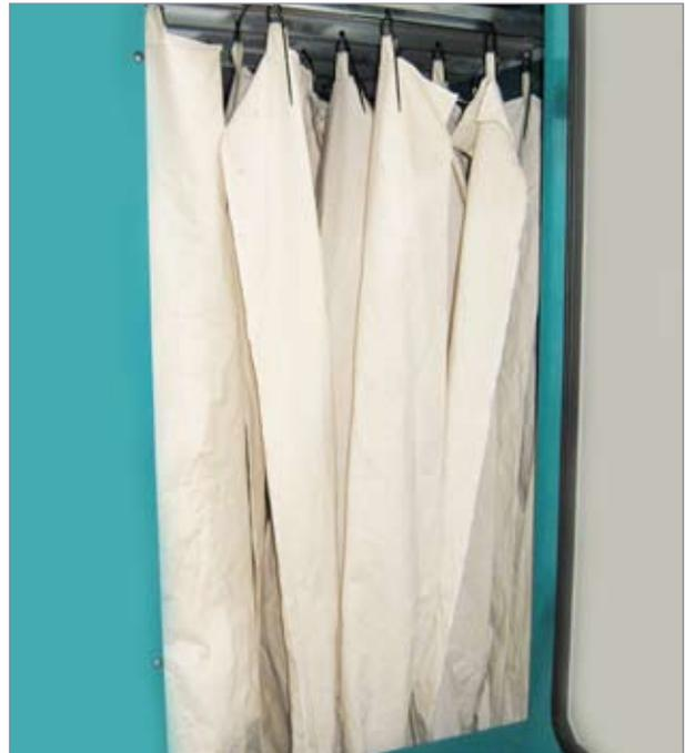
Check the 36 filters in the filter unit for damage and holes. When it is time to clean them, remove them and turn them inside out. You can then clean them with a high-pressure hose. Make sure that they are completely dry before refitting them.
