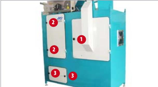
To open the doors, turn the handles counter-clockwise.
