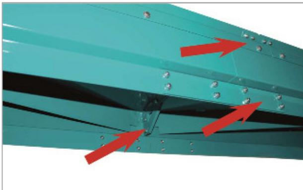
Conveyor belts over 6.0 metres in length are delivered in sections and assembled on site. Assemble the sections end-to-end and adjust such that the surfaces are level and in line. Attach six M8 bolts in the mounting plate inside the belt. Then attach the four reinforcement plates, two on each side. Repeat the above for each join between sections.
