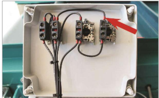
The conveyor belt is to run as a standalone unit with manual start and stop using the control Panel. The control line and input power must be installed on opposite sides of the start switch.
