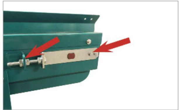
In order for the belt to pull and run straight during operation, it may be necessary to adjust the position and angle of the turn roller.
