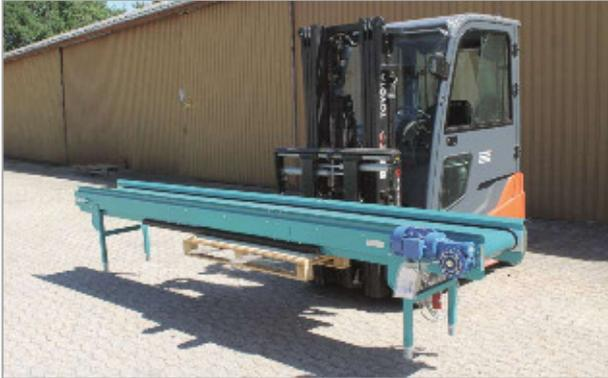
Conveyor belts 4.5 metres or less in length can be lifted under the centre.
