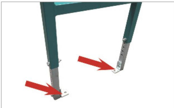
Conveyor belts over 6.0 meters long must be attached to the floor and adjusted so that each section above the legs is level and the entire length of the belt is in a straight line  $\pm 2$  mm. Conveyor belts less than 6.0 meters in length are not attached to the floor, but the sections must be adjusted so they are level.
