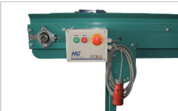
The machine must be connected to 3 x 400 volts with earth (PE), with a 16A fuse. Connect using a CE connector or a power isolator for safe disconnection when the machine requires maintenance or repair.
