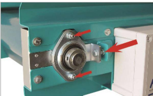
In order for the belt to run straight during operation, it may be necessary to adjust the angle of the pull roller.
