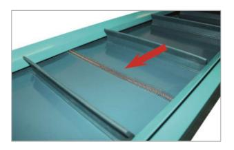
Run the belt through the sections. Hold the joints together and insert the joint strip. Fold the strip in over the belt and cut 10mm from the fold.
