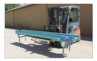
Conveyor belts 4.5 metres or less in length can be lifted under the centre.
