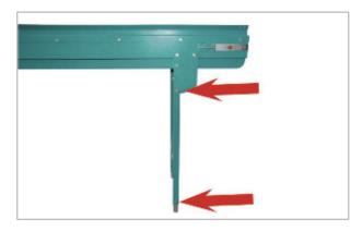
Lift the conveyor belt off the ground using suitable lifting equipment. Or lay it on its side before adjusting the legs.
