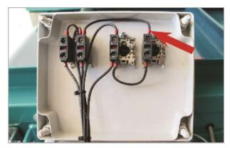
The conveyor belt is to run as a standalone unit with manual start and stop using the control Panel. The control line and input power must be installed on opposite sides of the start switch.
