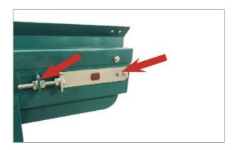
In order for the belt to pull and run straight during operation, it may be necessary to adjust the position and angle of the turn roller.
