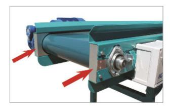
Remove the protective caps on the rollers at least once a week and clean underneath.
