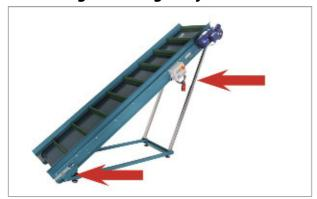
Adjustment of the low end of the conveyor belt depends on whether it is fitted with feet or wheels underneath.
