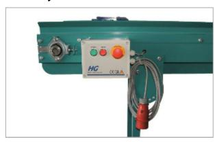
The machine must be connected to 3  $\times$  400 volts with earth (PE), with a 16A fuse. Connect using a CE connector or a power isolator for safe disconnection when the machine requires maintenance or repair.
