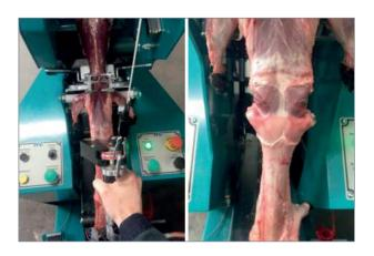
Press the fur pull pedal and pull it down to the eyes and apply a cut by the eyes.
