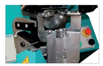
Place the tail section of the skin in the tail clamp. Make sure that no other body parts are between the jaws when the clamp is closed, as this will result in an unsuccessful pull. The leg skin clamp automatically captures the skin from the legs when the tail clamp is pulled up and over. Make sure that the clamp does not catch too much of the belly skin, as this risks tearing open the belly of the body/cadaver.
