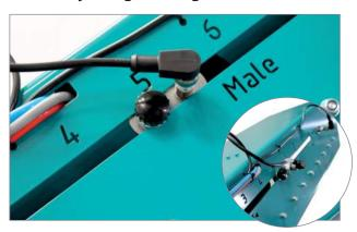
This sensor is used to define the length of the first pull before the machine starts to pull slowly. The sensor can be adjusted to ensure the machine runs slowly when it reaches the animal's shoulders. Move the sensor up if you are working with large animals, and move it down if you are working with small ones.
