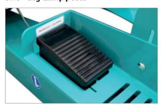
The pedal on the right-hand side activates the leg clamp used to secure the mink legs. Hold the pedal down until the skin-puller arm has passed the operator's knee. The pedal can then be released. If it is released earlier, the machine will stop.
