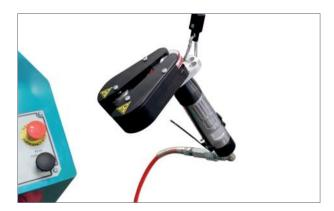
Use the head cutter to cut the skin free around the head. **WARNING!** The head cutter features rotating blades, so read the user manual carefully before use.
