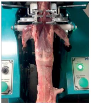
11 Use the decapitator to cut the fur free from the neck of the mink, make the first cut about 10mm above the dividing line by the ears.
