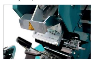
This is to place the mink's hind legs once the skin has been loosened on the HG Combi Cut or a different cutting machine used to loosen the hind legs from the skin.
