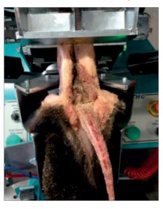
The leg clamp is now shut, let the animal hang loose in the leg clamp (the left pedal is still held down). Grab the tail skin from the animal with one hand, while the second hand pushes the tail clamp over the animal. While the tail skin is put in the clamp, the clamp closes automatically when it is pushed over the animal (watch out that your fingers do not get the clamp). The tail from the body may not get in the
