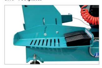
It is possible to adjust the height and angle of both right- and left-hand footplates. To do this, loosen the bolts and find the most ergonomic sitting position.
