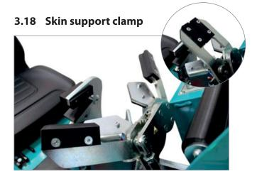
The skin support clamp helps to pull the skin when it has to be pulled down over the mink's shoulders. The clamp closes when the length sensor (3.16) is activated.
