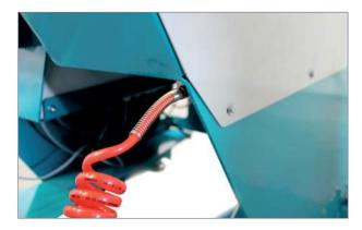
The connection can be positioned on the right- or left-hand side, as required. However, moving it from one side to the other requires remodelling other parts of the machine.
