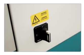
The main switch must be <ON> before the machine can be used. **WARNING!** You MUST disconnect and lock the main switch in its <OFF> position before starting any maintenance work.
