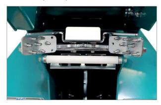
The body clamp secures the mink's body when the skin is pulled down over the head and cut free. To activate the clamp, use the two green buttons on the right- and left-hand panels. The clamp must be activated when the cadaver shoulders are placed in the clamp.
