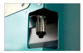
The mist lubricator ensures that the head cutter is lubricated properly, runs optimally and lasts longer. Remember to fill the mist lubricator container regularly with mist lubrication oil.
