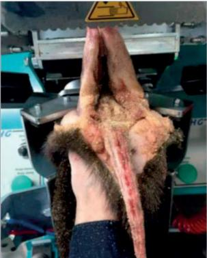
The leg clamp is closed by pressing the left pedal and holding it down. If the legs are not placed properly in the clamp, release the pedal and the clamp opens again.
