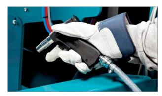
After finishing work, check the machine for foreign objects that may have been caught in it. Use a compressed air pistol to remove wool and dirt from the machine parts. Use compressed air to remove any dirt from the motors' radiator fins. Use a vacuum cleaner to remove dust and wool from the floor around the machine. Regularly check the surfaces of the fan/motors for dust and other impurities. If the layer of dust is more than 0.5 mm thick, it must be removed.
