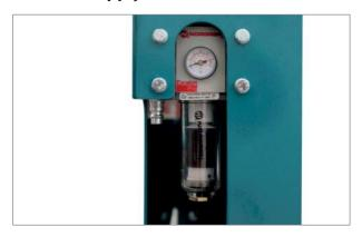
Connect the air supply here and make sure the pressure is at least 7 bar. Check regularly to make sure the fine filter is clean and that the machine receives air at a pressure of at least 7 bar. The maximum permitted pressure is 9.5 bar. Pressures higher than this may damage the machine valves.
