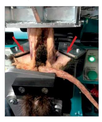
When the slow pull is activated the adjusting is done by moving the sensor on the side of the body cover. The sensor is activated when the leg clamp runs up past the sensor. The sensor makes the machine pull slowly. The support of the clamp for the skin closes and the leg skin clamp opens. Adjust the sensor so that it will slow down just before the skin is pulled off to the shoulders of the animal.
