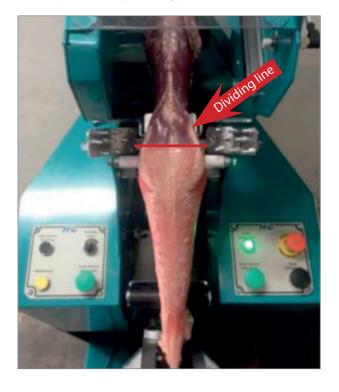
8 If the dividing line is not in the center of the clamp after the pull, then you can either increase or decrease the fur pull speed.
