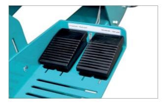
The pedals on the right-hand side control the skin and body pullers. They can be activated separately or simultaneously.
