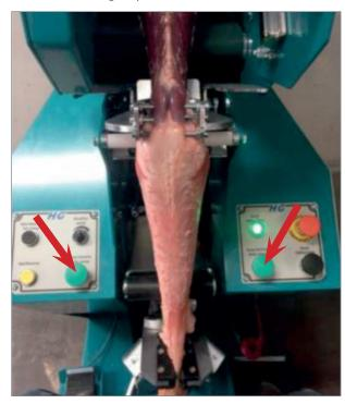
10 Continue pressing on the pedal for fur pull until the skin is pulled down over the shoulders to the head.
