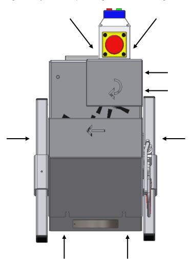
When you clean around the brushes, first disconnect the electric and the air connection. Dismount the bolts by the 8 marks and remove the screens.
