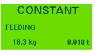
**Constant**: Press the CO Button. The pump will start and run until the CO Button is pressed again. The counters will update when the pump is stopped.
