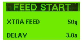
Feed Start: Used to compensate for pressure loss in the feeding pipe between stops. Xtra Feed (10 to 500gram). Delay (the time the pedal is released) (1 to 10 seconds). The function is on when the blue light is shown. Choose by pressing the menu button, change value with up/down buttons. Press enter to return to operational screen.
