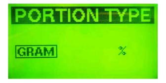
Press menu and Portion Type will appear, choose between gram and % with the menu button select with enter. When the top line is highlighted, use arrow up to reach next menu. The minimum amount to ad is 5 gram.
