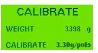
The screen shows weight and amount of feed for each signal from the sensor for a short while. Then it changes automatically to the startup screen.
