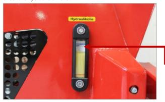
**WARNING!** Fit the tipping protection. Top up with type Q8 Handel 46 hydraulic oil or similar, if necessary.
