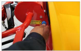
The coasting button is used to disengage the drive wheels, allowing the motorised wheelbarrow to be moved when the engine is off. Turn the button counter-clockwise to disengage. Push the button and turn clockwise to re-engage the engine.
