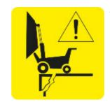
Do not operate and unload the motorised wheelbarrow near excavations and unstable edges.
