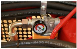
The indicator gauge on the hydraulic filter indicates whether the filter needs servicing or replacing.
