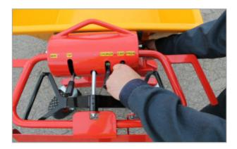
Start the machine by activating the choke when the engine is cold and then turning the ignition key clockwise. When the engine is running, release the key and adjust the choke until the engine is running smoothly. Adjust the throttle to the desired engine revolutions.
