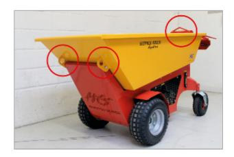
Ensure sufficient stability during lifting to prevent disconnection.
