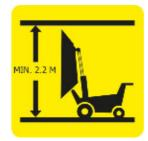
The machine may only be transported using a vehicle with sufficient headroom as there is a risk of serious injury and damage to the operator, machine and transport vehicle.
