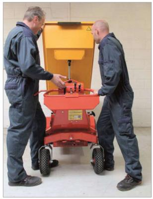
In case of an engine fault, the tray can be tipped manually. This task requires two people.
