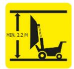
Do not operate the motorised wheel-barrow at insufficient ceiling heights.
