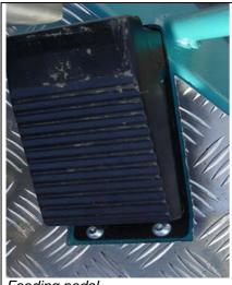
Feeding pedal is placed outer right on the machine.
