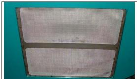
Particle filter oil cooler
