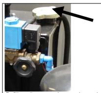
Refill cooling water / expansion tank.
