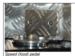
Speed (food) pedal is placed on the right side, between the feed pedal and the central bracket.
