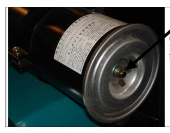
Cleaning/change of air filer. Remove the wingnut in the end of the air filter house, and pull out the filter.
