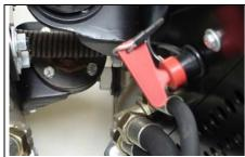
The main switch is placed at the back of the fore carriage.
