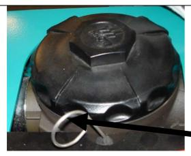
You refill hydraulic oil by removing the big screw cap.
