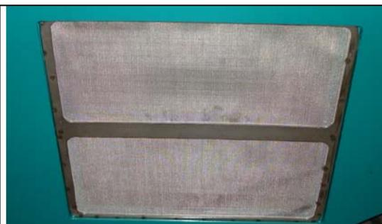
*Particle filter oil cooler*
