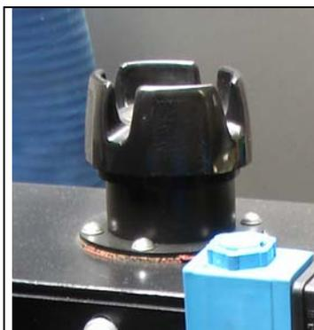
Unscrew the filler cap and refuel with diesel oil.
