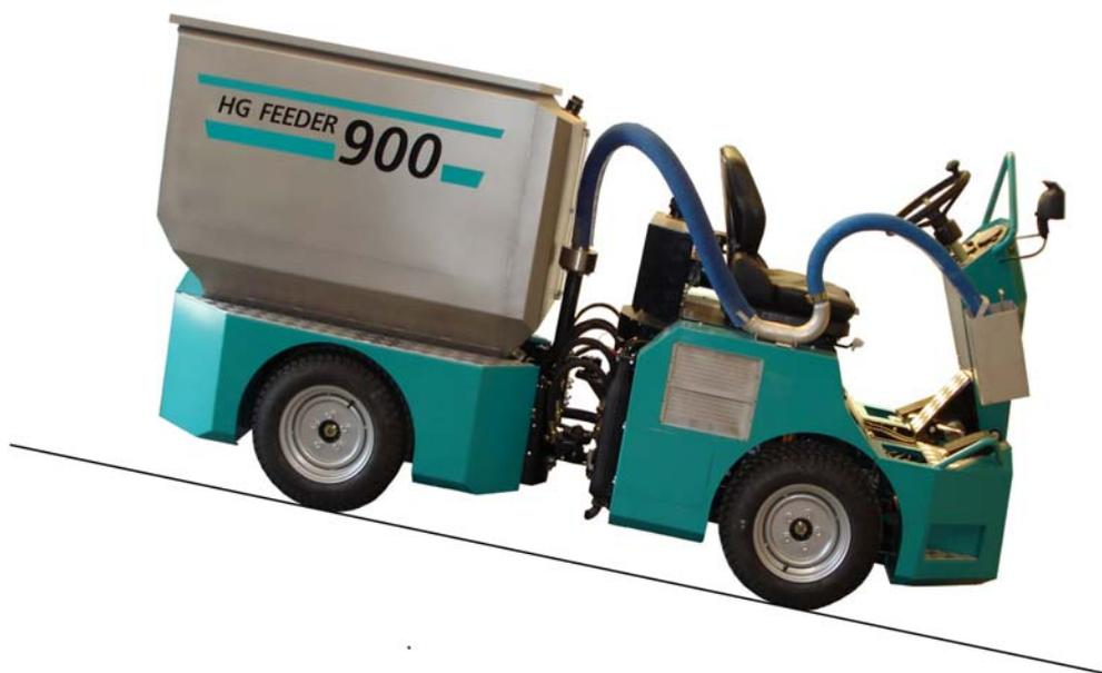
*Never park on a sloping foundation, the machine will run!*
