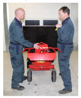
In case of an engine fault, the tray can be tipped manually. This requires two people. There must be a person on each side of the machine's handle bar. Push up the tipping lever while simultaneously pushing up the tray.
