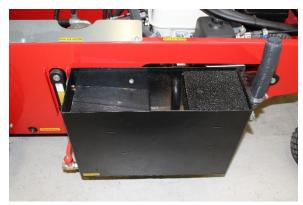
Remove the cover on the filter box and clean the filter using warm water.
