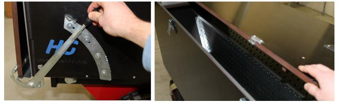
Check that the emptying hatch and top latch seal properly by opening and closing the latch. Check that the seals are intact and seal correctly. Close the handle for the emptying hatch and the top hatch hasp securely.
