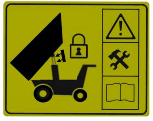
**WARNING:** Always mount the safety fittings for the tipping cylinder before starting the inspection work.
