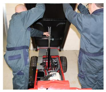
While one person holds up the tray, the other mounts the safety fitting on the hydraulic cylinder.
