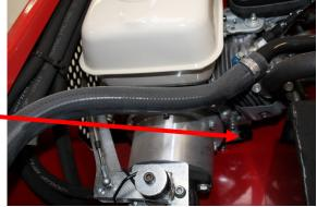
Top up with type 15W-40 engine oil, if necessary.
