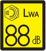
When tipping with an empty tray and maximum revolutions, the highest energy-equivalent sound pressure level at the operator's position has been measured at 88 dB (A) in accordance with ISO 6396.
