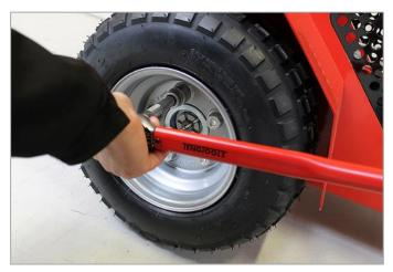
Retightening the wheels Retighten the wheel nuts once a week. Torque: 100 Nm
