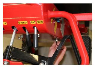
Start the machine by activating the choke when the engine is cold and then turning the ignition key clockwise. When the engine has started, release the key and adjust the choke until the engine is running smoothly. Adjust the throttle to the desired engine speed. The choke should be fully deactivated after a while. If the engine is warm, it is not necessary to use the choke.
