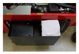
If further filtering is required, place a cotton cloth on top of the filter.
