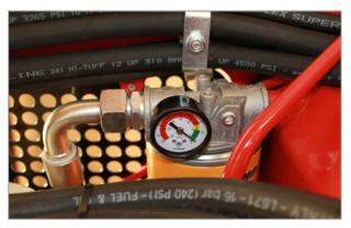
The indicator light on the hydraulic filter indicates whether the filter needs servicing or replacing. Apply full throttle, and check the indicator light. If the needle is in the red area, the machine needs servicing.
