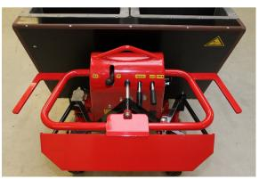
Pressing the safety plate should move the machine forward, preventing the operator from being trapped during reverse.
