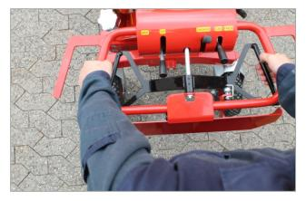
Place both hands on the handle bar so that your fingers can reach the forward handle. Pull up the hand lever on the right to move the machine forward and release to stop. Pull up the hand lever on the left to reverse.
