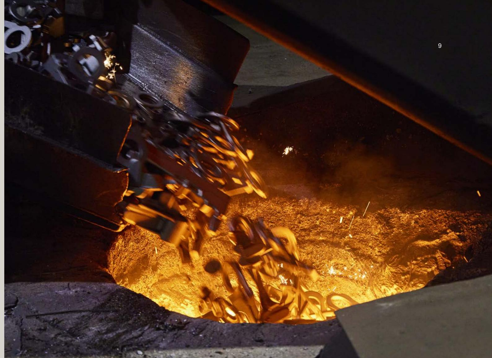
For BIRN in Holstebro to produce and deliver around 47,000 tonnes of cast iron each year, approx. 90,000 tonnes of iron must be melted. Much of this iron comes from scrap metal and recycled foundry returns. Foundry returns refer to running systems and feeders.
