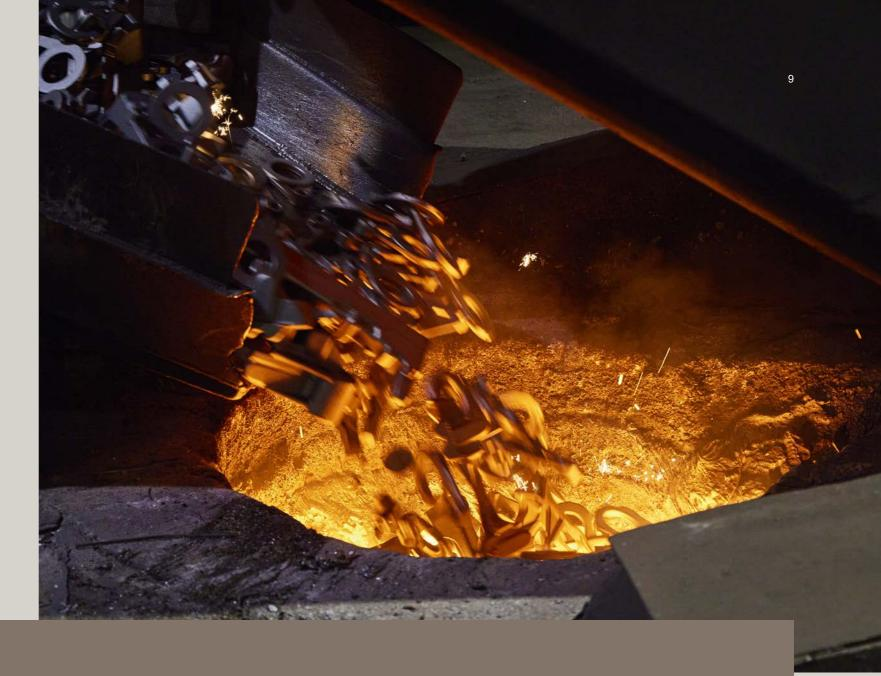
For BIRN in Holstebro to produce and deliver around 47,000 tonnes of cast iron each year, approx. 90,000 tonnes of iron must be melted. Much of this iron comes from scrap metal and recycled foundry returns. Foundry returns refer to running systems and feeders.
