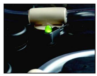
Battery Watering Monitor - otherwise known as the "Blinky" (because it blinks!). The Blinky is a probe that is inserted into one cell of a battery. It has a flashing green LED that informs battery maintenance personnel when the battery needs water, and when it does not, as follows:
