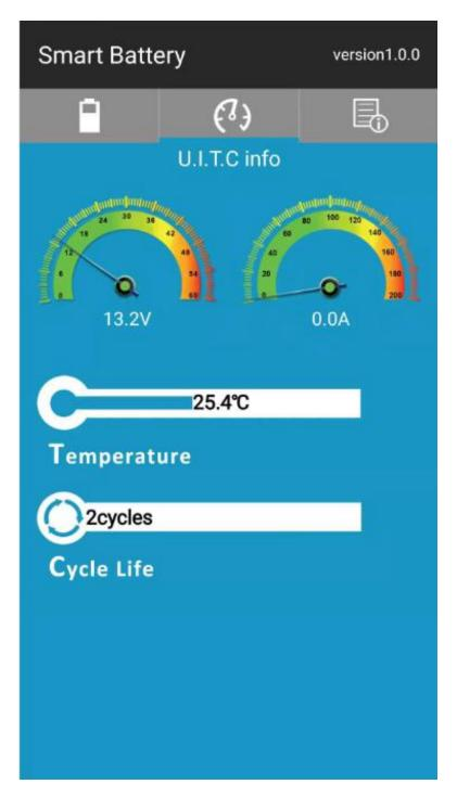
U.I.T.C means voltage, current, temperature and cycle life, all details shown in real time.
