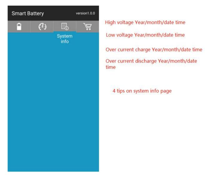
System info will show high voltage, low voltage, over current charge, over current discharge.
