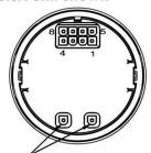
USED FOR DEVICE CONFIGURATION DO NOT CONNECT WHEN INSTALLING GAGE
