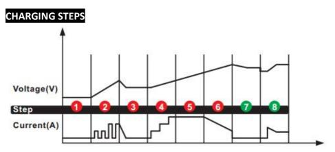
**STEP 1: DIAGNOSIS** (Check if battery has connected with the charger and also check battery voltage)
