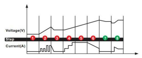
**STEP 1: DIAGNOSIS** (Check if battery has connected with the charger and also check battery voltage)
