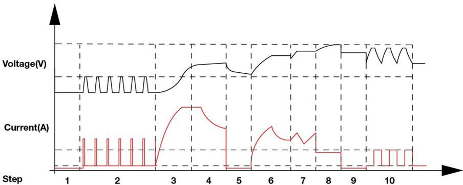
**STEP 1: ANALYSING 1** (Checks if battery has connected with the charger)
