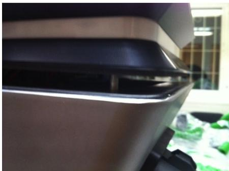
2. Lift the bottom cover up to the mounting frame.
