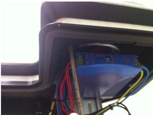
5. Disconnect eventual antenna cable connecting top cover with frame and remove the top cover
