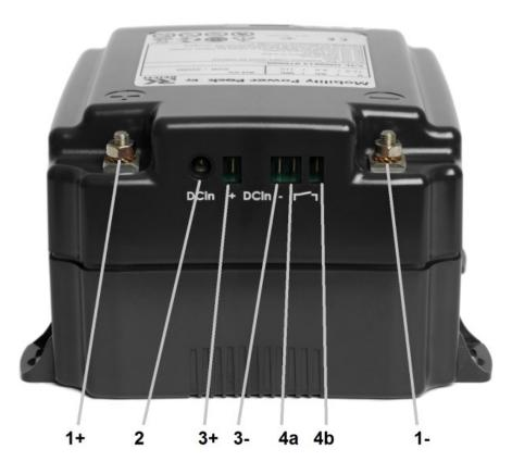
(1+) (1-) Mount the caravan mover plus and minus cables at the output terminals with M6 nuts. Beware the correct polarity.
