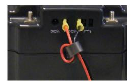
(4a) (4b) An external push button can be connected to the terminals at r'r This external push button has the same function as the internal push button near the LEDs (switch on/off and clearing an error).
