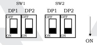
Only the set of dipswitch SW1 (the one on the left side) has effect on charging curve selection accordingly to the table above.
