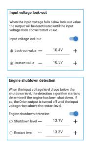
(*Re)start level:* The default setting (13.3V) is based on generic smart alternator setup. Most smart alternators will generate 13.5V when the engine is running, and regular alternators will normally generate >14V. In an application with a regular alternator the restart level can therefore be set to a higher value, e.g. 14V.
