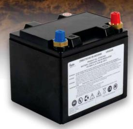
The inherent design of the VRLA Armasafe battery minimises gas evolution and eliminates the need to top up periodically with water. The electrolyte is fully absorbed into the glass mat separators between the positive and negative plates, which mean there is no free acid within the battery case; this gives increased flexibility in mounting position.
