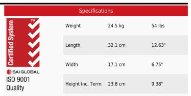
Product measurements & weights are calculated based on sample data. Individual specifications are subject to vary due to the manufacturing process, battery components & electrolyte levels.
