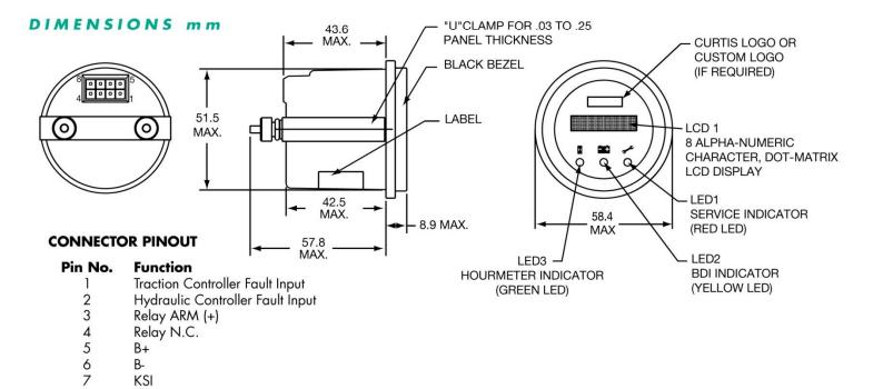
**Note**: In addition to a "U" clamp and thumbnuts/washers shown in the drawing, individually packed units are provided with a mating connector and female pins. Bulk packed units are provided with a "U" clamp and hex nuts/washers only.
