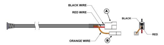
Connect (A) to the battery or caravan board system with one of the two included connection cables. Red is positive (+) and black is minus (-).
